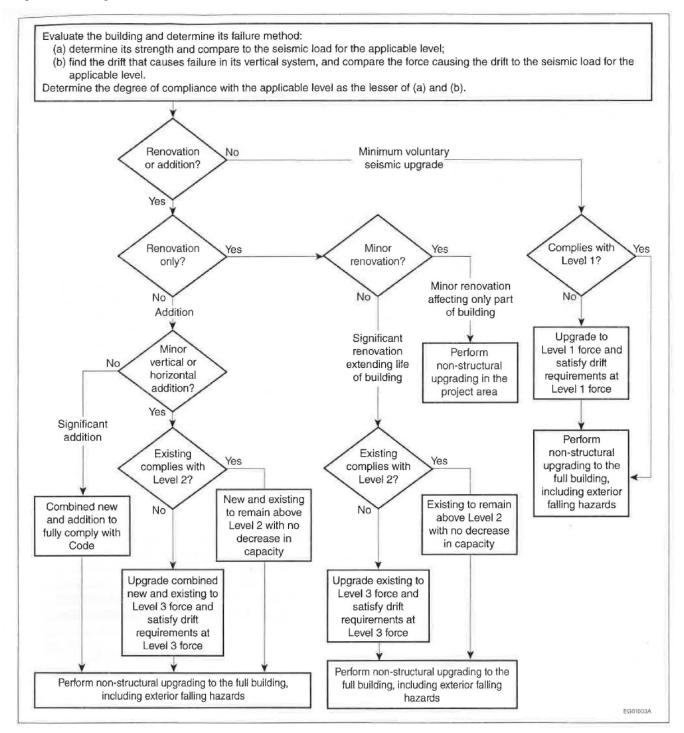
Figure 2. Upgrading Flowchart.
